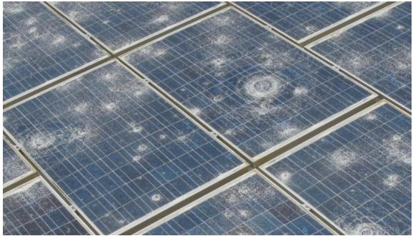
Figure 7 – Examples of hail damage on PV modules
