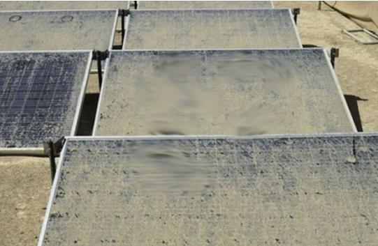
Figure 6 - Effect of sand deposit after sandstorm
