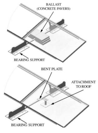
Figure 1 – Ballast only PV System
