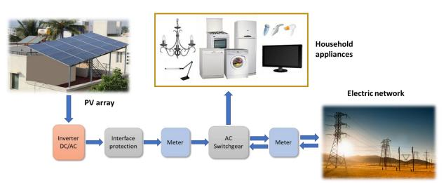
Figure 3 – Block diagram of a grid-connected solar PV plant for a household
