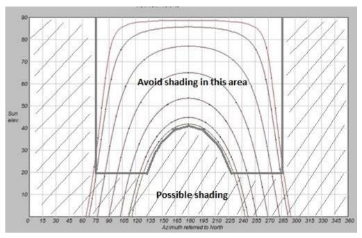
Figure 2 – Solar paths and recommended maximum shading
