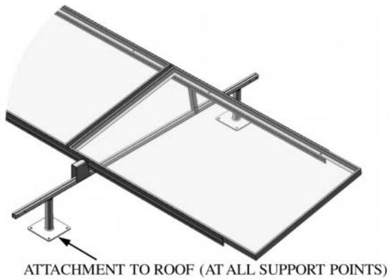
Figure 3 - Structurally attached on flat roof PV system
