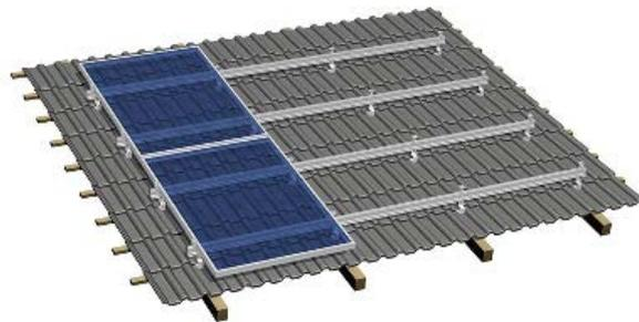
Figure 4 – Structurally attached on tilted roof
