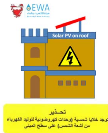
Figure 2 – Example of a warning, which indicates the presence of solar PV plant with possible hazardous voltage
