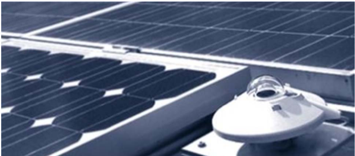
Figure 6 – Example of an in-plane pyranometer
