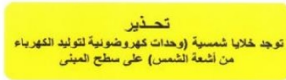
Figure 10 – Sign to be used to indicate the presence of a PV plant
