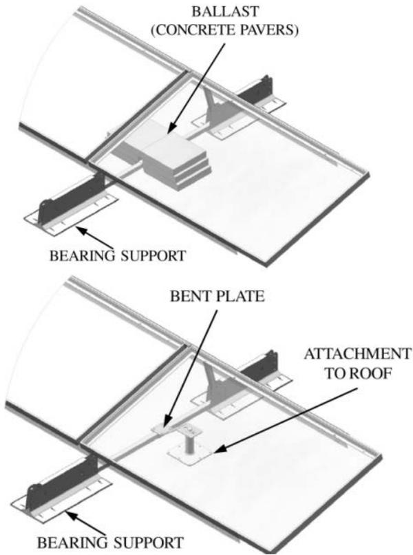
Figure 1 – Ballast only PV System
