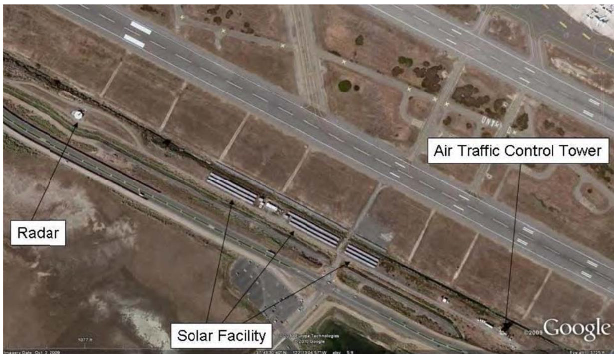
Figure 11 – Ground mounted PV panels at Metropolitan Oakland Int. Airport – California (source: [4])
